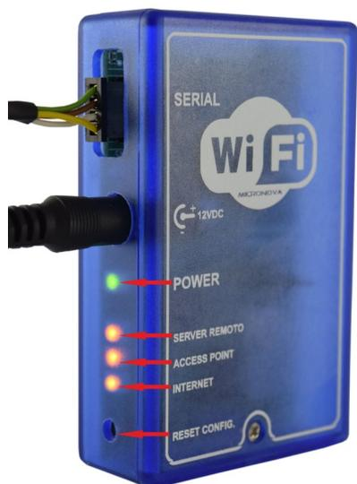
1. Connect the Wi-Fi module to the electric mains through the power supply included in the KIT.
